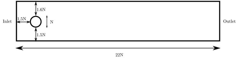
Figure 13: Geometry for the flow past a cylinder.
