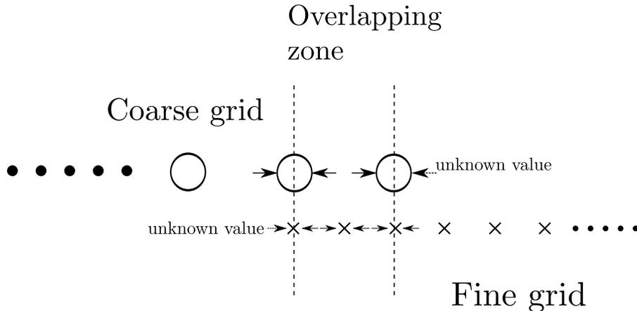
Figure 5: Overlapping zone between coarse and fine grids
