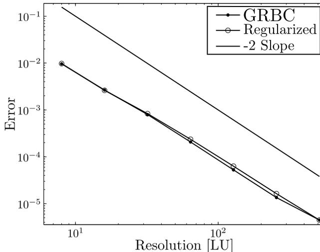
Figure 5: (Numerical accuracy in a 3D channel flow. The error curve of the Regularized BC is also present for comparison purpose.
