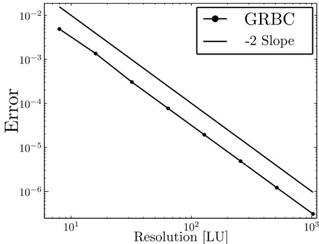
Figure 3: The error of the Womersley solution with respect to the resolution in lattice units.
