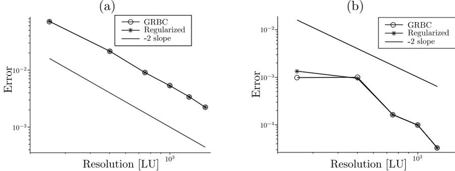
Figure 4: Numerical accuracy in the 2D dipole-wall collision flow for the two enstrophy peaks, (a)  $\omega_1 = 933.6$ , and (b)  $\omega_2 = 305.2$ . The error curve for the enstrophy peak obtained with the Regularized BCs also added for comparison purpose.
