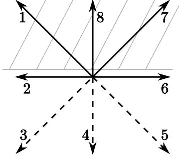
Figure 2: A boundary node for the D2Q9 lattice. The dashed arrows represent the unknown populations.
